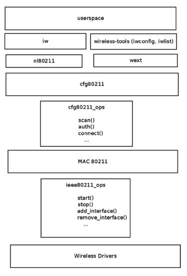
Figure 12-5. Linux wireless architecture
