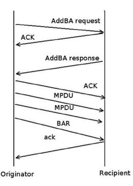
Figure 12-7. Immediate Block Ack
