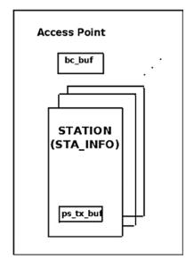
Figure 12-3. Buffering packets in an AP
